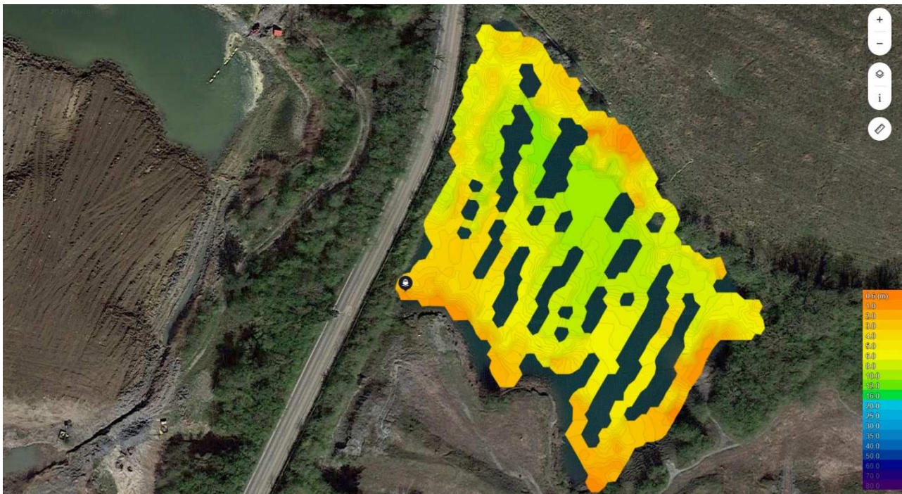
Figure 45 Blue Pool bathymetry data processed at high resolution, overlaid over a satellite map (Google) and colour coded to show shallow depths in orange and deeper areas in green. Gaps in the dataset are apparent.
