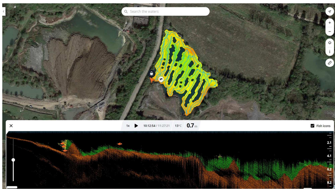
Figure 36 Blue Pool bathymetry data showing the route of the kayak across the water (blue line overlaying the map) and a depth profile (insert below).
